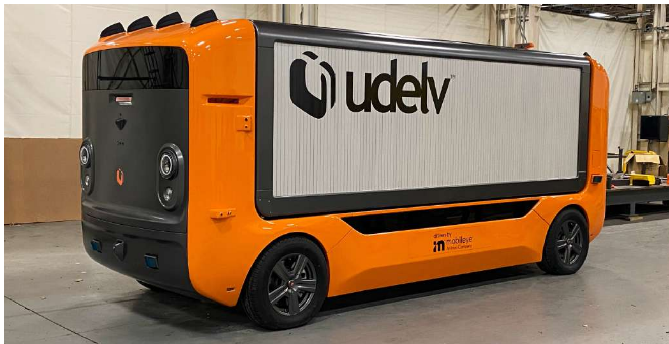
The autonomous Udelv Transporter's uPod can carry up to 2,000 lbs. of cargo and make up to 80 stops per run.
