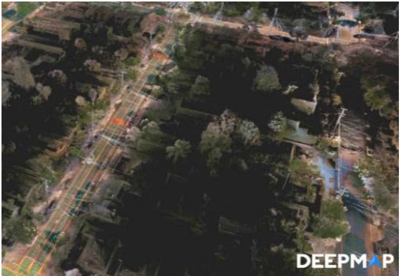
A DeepMap map in San Jose, Calif., depicting highly detailed features of the road and surrounding city block environment, including a reliable semantic layer of information with key attributes such as navigable boundaries, lane boundaries, crosswalks, traffic signs and traffic signals, explicit and implicit yield lines, and lane connectivity.
